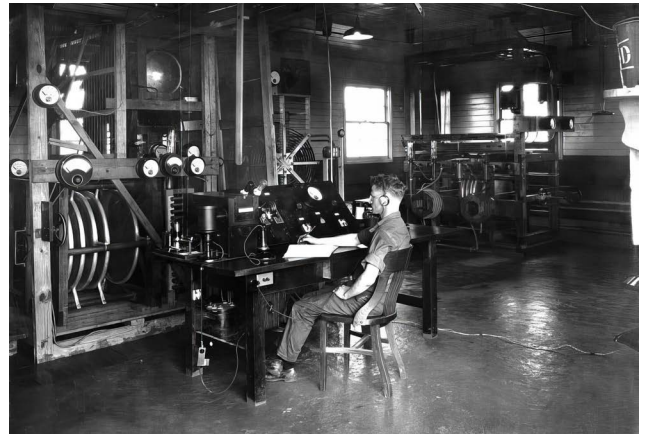
This is an early view of the General Electric radio laboratory in 1925, showing an experimental 109-meter transmitter (2,750 kHz).
