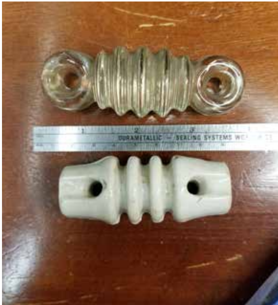
Insulators used to construct wire antenna are available made from glass, porcelain, or plastic (not shown)
