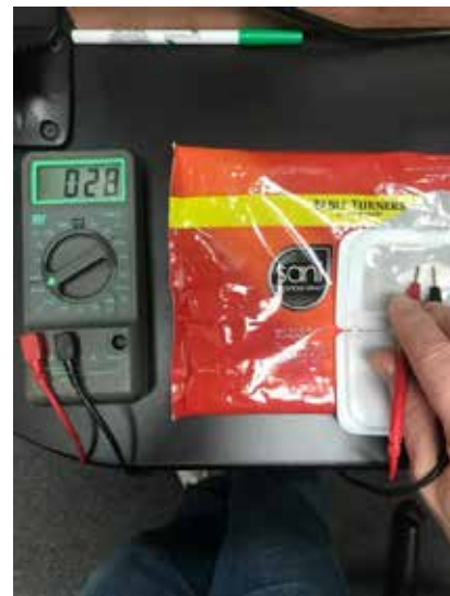
Fig. 1: Cleaning wipes may be conductive, posing a risk to electronic parts.
