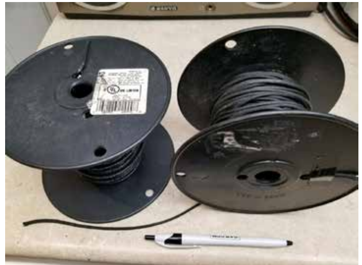
THHN wire and polyester antenna support rope are available in 500 foot spools
