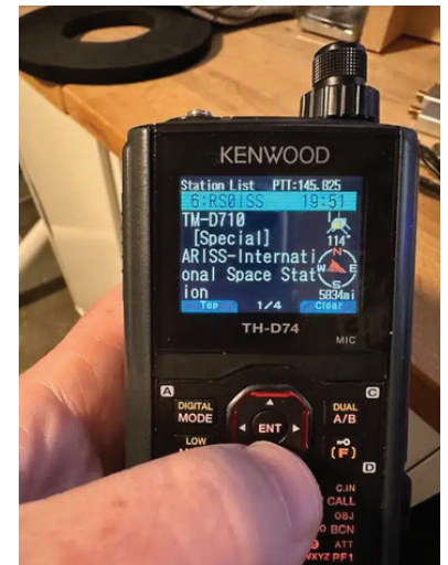
A Kenwood TH-D74 displays a packet received from the ISS, which uses the call sign RS0ISS for its APRS radio.
