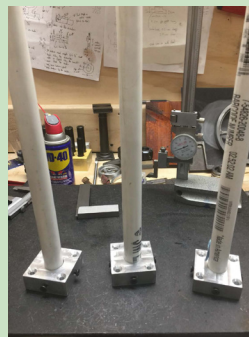
Aluminum blocks drilled and tapped. The PVC pipe stand-off fits in the center and the outer holes allow for mounting to the side of the house.
