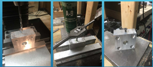
Aluminum blocks drilled and tapped. The PVC pipe stand-off fits in the center and the outer holes allow for mounting to the side of the house.
