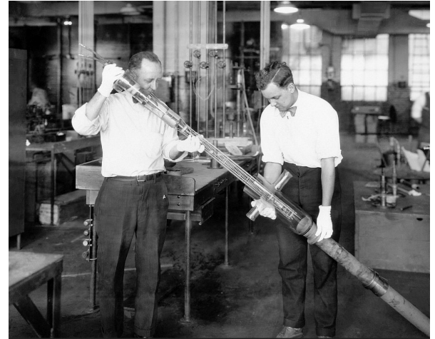
Assembling a 100 kW UV-862 tube
