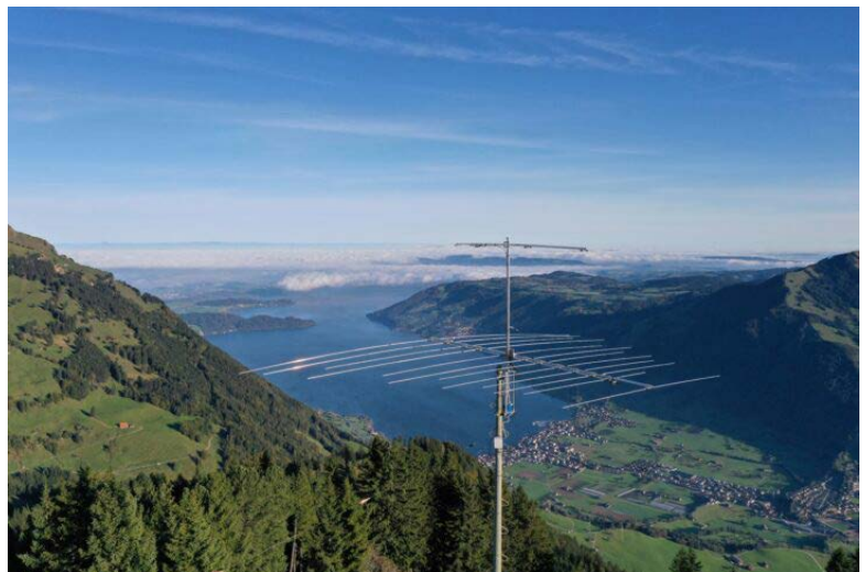
A mounted Optibeam OB9-5 antenna monitors the 10m, 12m, 15m, 17m and 20m radio bands, anchoring the remote listening setup on Mount Rigi in Switzerland.
