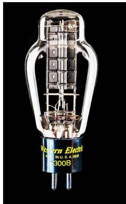
A delicate 15-inch ribbon of nickel makes up the filament at the heart of Western Electric's current model, the 300B
